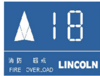
LCL-DP02 Segment code display in elevator cab
